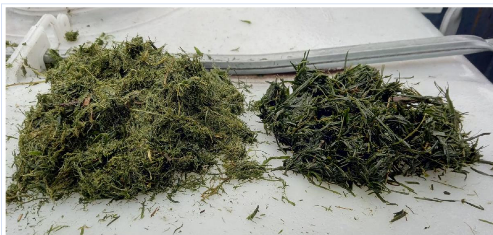
Figure 3. Left: Grass fiber fraction after treatment in Twin Screw Press. Right: Fresh grass after treatment in Seko mixer.
